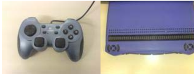
Figure 5: The Logitech controller (left) and the Braille display (right) which are used for the second bimanual interface
