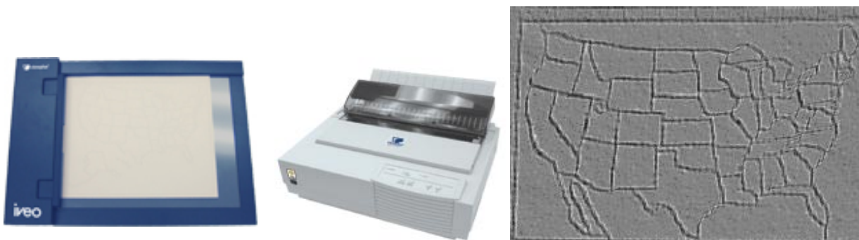
Figure 6: To the left the IVEO TouchPad, in the middle the Cub Braille printer, and to the right a tactile printout of the USA map to be placed on the TouchPad.
